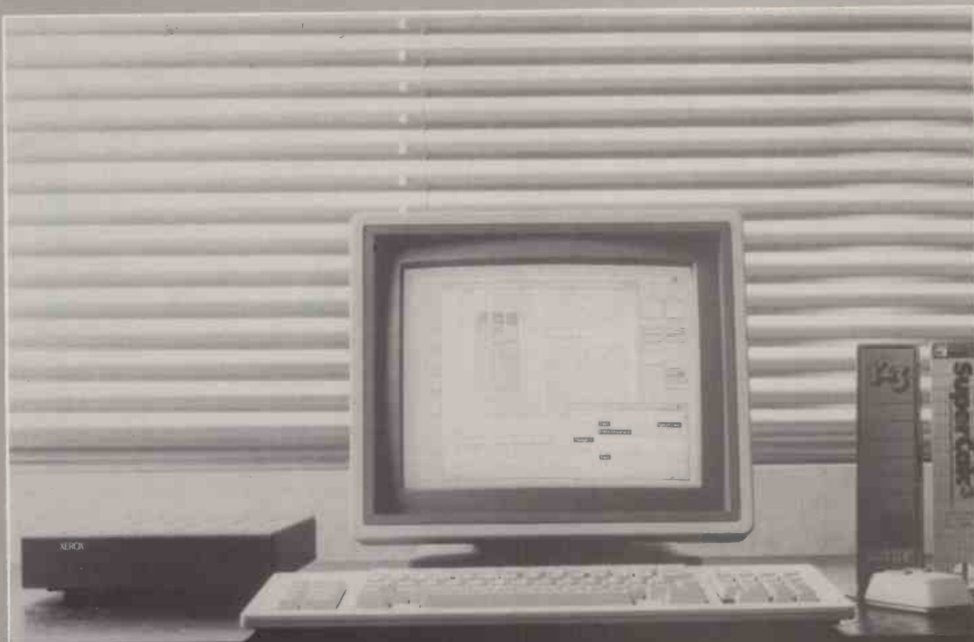
Left: The 6085 PCS emulating an IBM PC with four floppy discs and an 80-column colour display; in reality we had a hard disc and one floppy.
